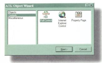
Figure 4 – The ATL Object Wizard lets you add new object types to an existing ATL project. Here, we've chosen the Control page and we're about to add a new ActiveX control to the project.
