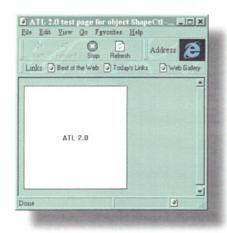
Figure 5 – Here's the initial, 'do-nothing' control running inside Internet Explorer. The initial drawing code (the bit that announces ATL 2.0) is automatically included by the ATL Object Wizard.
